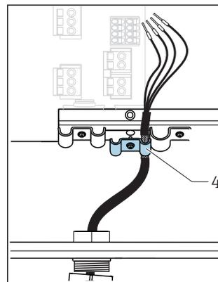
▣ 29 Inserting the cable
