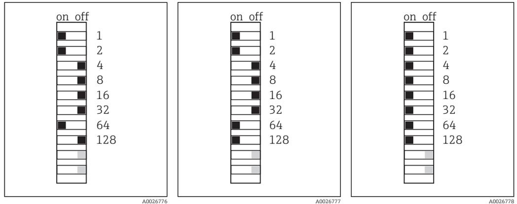
70 Valid PROFIBUS address 67 71 Valid Modbus address 195 72 Invalid address 255 <sup>1)</sup>
