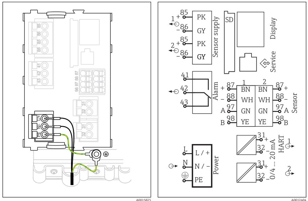
31 Connecting power supply on the BASE-H or -L 32 Overall wiring diagram for BASE-H or -L
