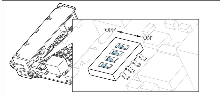
68 DIP switch for internal termination
