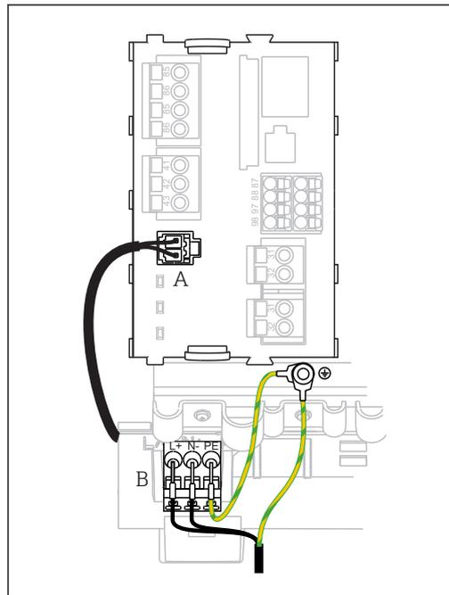
34 Power supply connection on the BASE-E
