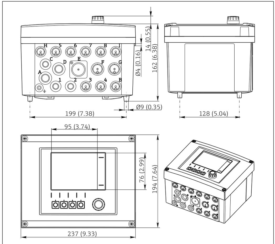
6 Dimensions of field housing in mm (inch)
