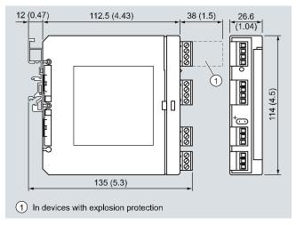
Dimensions for control room mounting, rail mounting in mm (inches)
