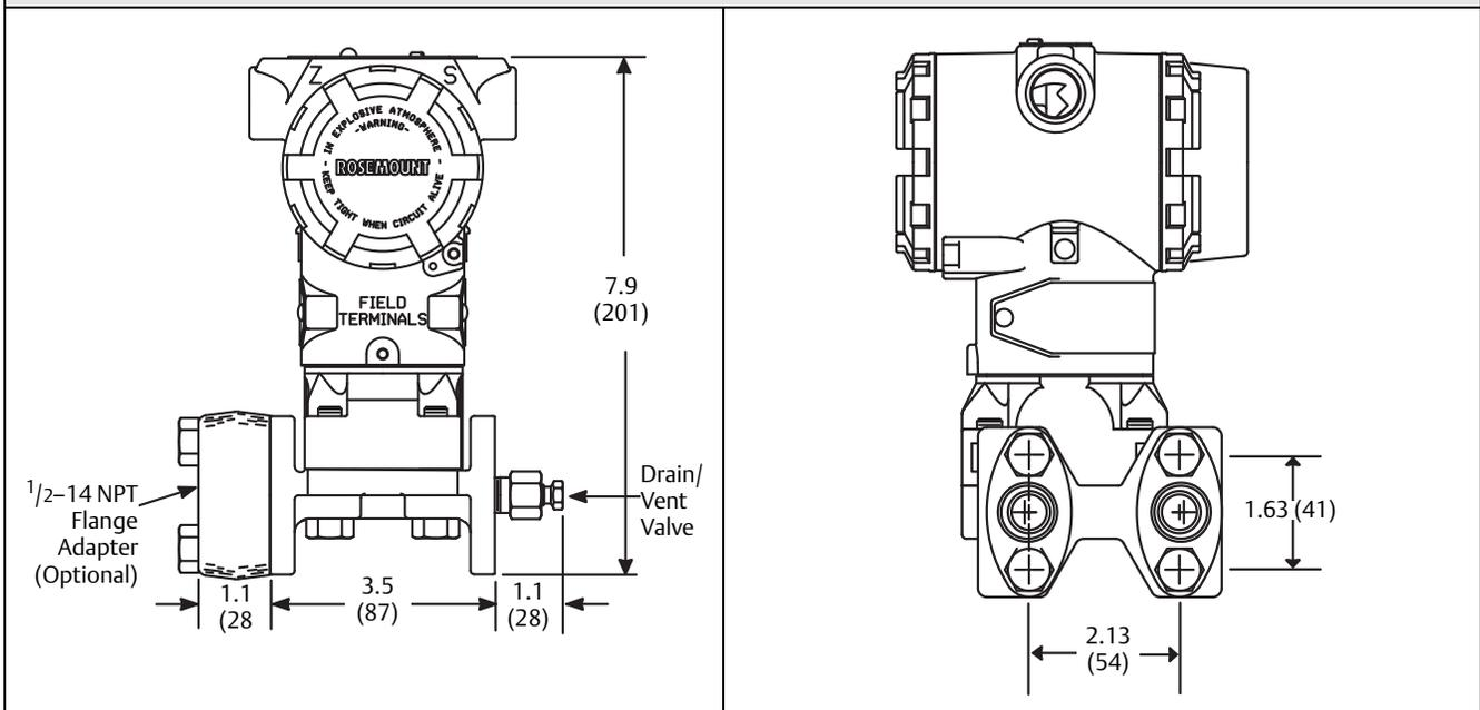
**Standard 3051C Coplanar with Rosemount 305 3-Valve Traditional Integral Manifold**
