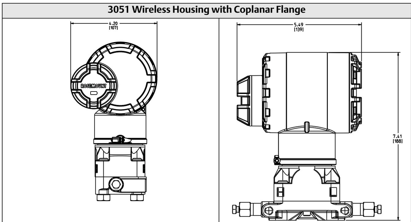
**Standard 3051C Coplanar Flange with Rosemount 305 3-Valve Coplanar Integral Manifold**
