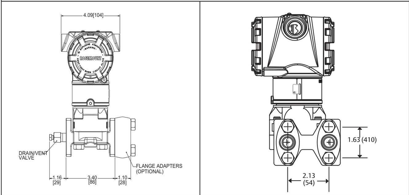
**Enhanced 3051C Coplanar with Rosemount 305 3-Valve Traditional Integral Manifold**
