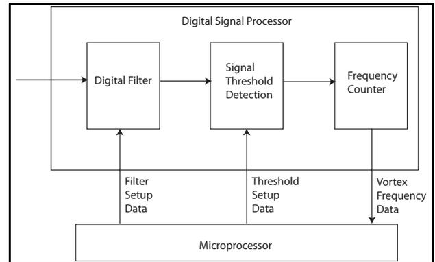
Signal-threshold detection is carried out via comparison of the digital filter outputs to the trigger level. This section facilitates rejection of sub-threshold noise and acceptance of the above-threshold signal.
