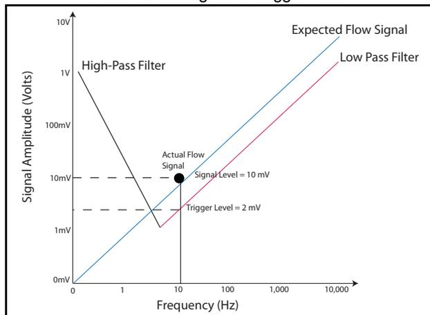
Figure 15 illustrates the signal strength measurement of signal-to-trigger ratio. In this example, the flow measurement frequency of 10 Hertz (Hz) has signal amplitude of 10 millivolts (mV). The threshold limit or trigger level of the filters at a frequency of 10 Hz is set at 2 mV. This means the signal-to-trigger ratio is 5 ( $10 \text{ mV} \div 2 \text{ mV} = 5$ ).
