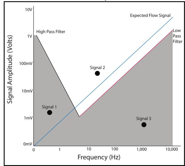
Figure 5 illustrates how the filters work to measure the flow signal (Signal 2) and reject noise signals (Signal 1 and Signal 3). Only signals in the non-shaded region will be accepted as flow signals. Signals in the shaded region will be rejected as noise.
