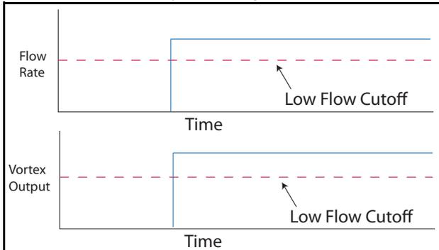
Figure 13 shows the flow rate starting at zero and then making a step change to a flow rate that is greater than the Low Flow Cutoff setting. With the LFC Response Type set to stepped, the output will jump to the measured flow rate value once the measured value is above the Low Flow Cutoff setting.
