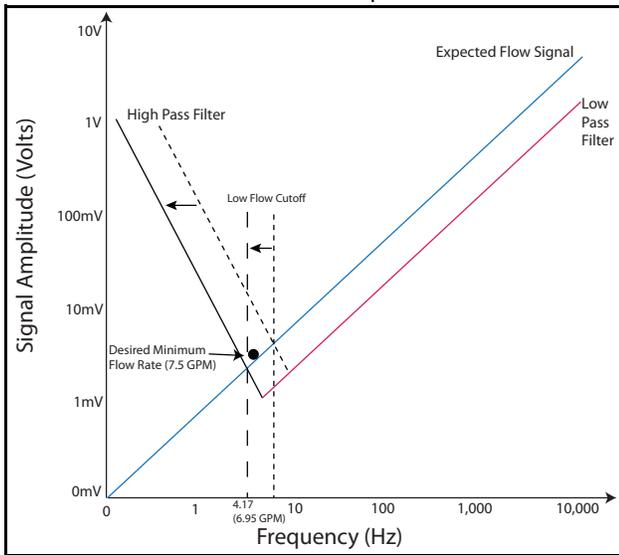
Figure 23 shows the filter settings with the low flow cutoff adjusted downward below the desired minimum flow rate. As stated in “Low Flow Cutoff” on page 13 the low flow cutoff can be adjusted in 18% steps. In this example, two steps of adjustment were required. A third step may be desired to allow for the 18% dead band around the low flow cutoff. The goal of adjusting the low flow cutoff is to allow the desired minimum flow rate to be measured without letting in additional noise.
